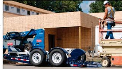
The 4 degree load angle is ideal for low ground clearance or reduced gradeability equipment.
