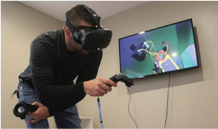
Training provider Interplay Learning uses virtual reality technology (shown in the image) to enable hands-on skills development in an interactive learning environment. Point-of-view simulations, either online or in virtual reality, put a user in a service call scenario, where an HVACR technician must learn in an environment that mimics the real world.
