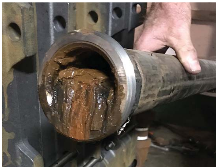
The sludge has accumulated at the return connection to the boiler.
