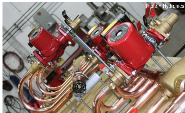
Circulators in a hydronic heating panel ready to ship to the job site.
