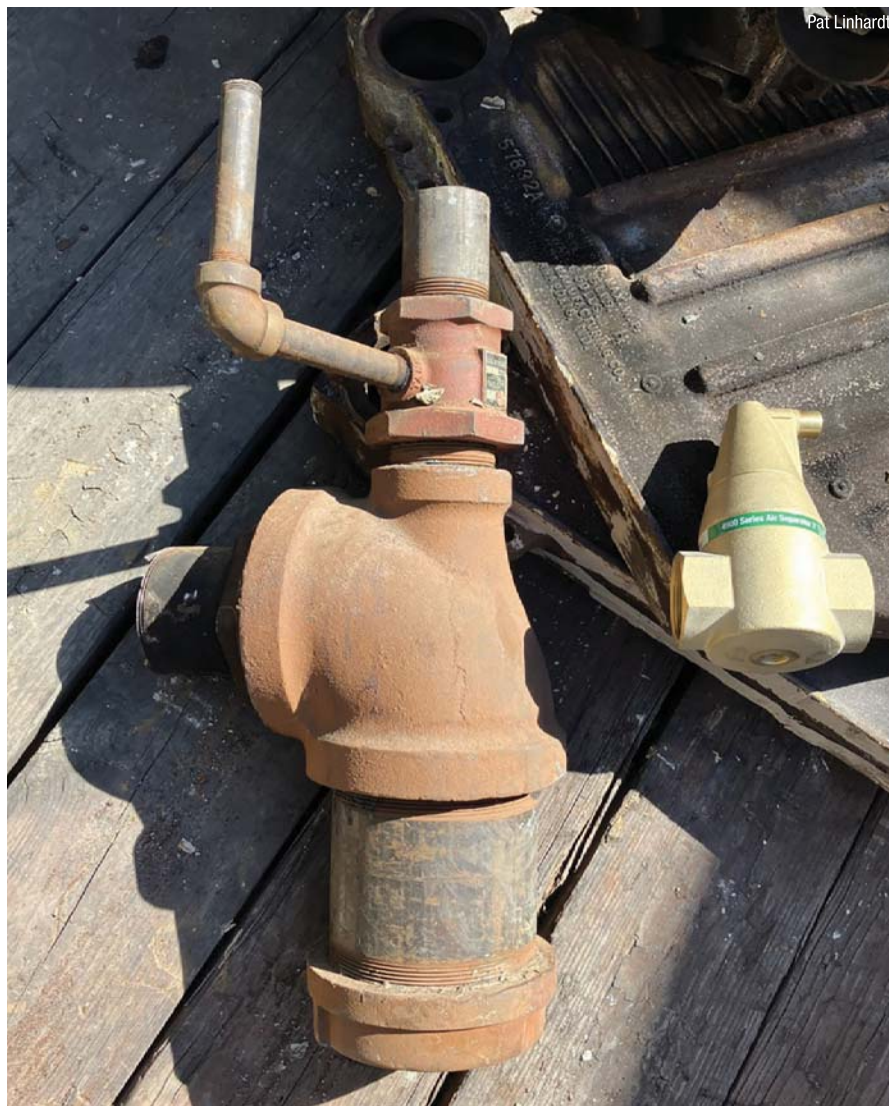
The red fitting on top of the very large tee is a Bell & Gossett dip tube air separator.
