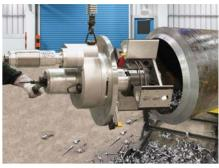
**THE DICTATOR II MILLHOG PIPE BEVELER** from Esco Tool is an I.D.clamping, welding-end prep tool that aligns perfectly using self-centering clamps. It can incorporate four blades in order to bevel, face, and bore or create a compound bevel. Featuring an adjustable tool post for easily indexing the blades, it can perform 37.5° to 10° compound bevels on a 24" O.D. pipe with a 2"-thick wall. *Esco Tool*
