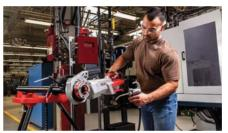
▲ THE 760 FXP POWER DRIVE CORDLESS THREADER is the first hand-held cordless threading solution designed for portability and ease of use. The 760 FXP threads faster than any other cordless hand-held threader on the market today when threading 1½" to 2" Schedule 40 pipe. *RIDGID* WWW.RIDGID.COM
