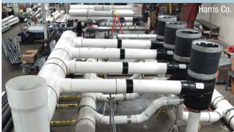
A large prefabricated piping assembly for the Minneapolis Bus Garage job. Note the worker in back for scale.
