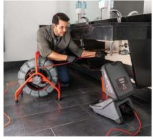
▲ SEESNAKE MINI PRO INSPECTION CAMERA from Ridgid features TruSense technology, best in-pipe image, navigation flexibility and digital zoom/pan for enhanced traceability. It is designed to inspect up to 200' of 1½- to 8" pipe with its midflex push cable that can navigate hard 90° bends. The 25 mm digital camera is self-leveling.
