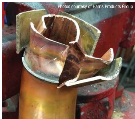
Skipping any of the basic brazing steps can lead to pipe joint failure.
