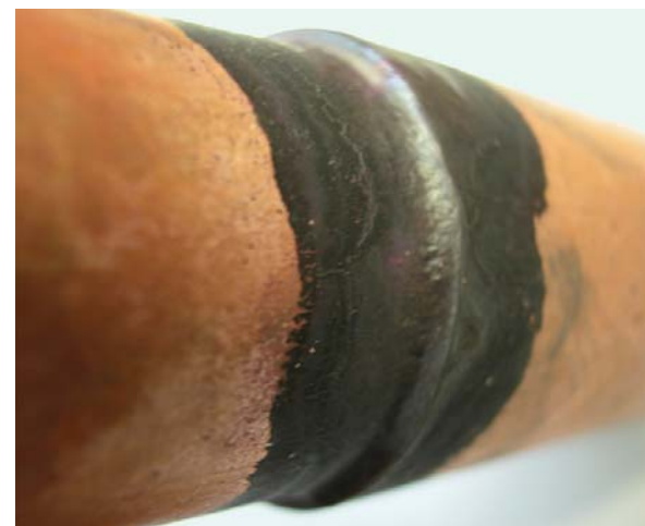
A quality brazing job results in strong, long lasting pipe joints.
