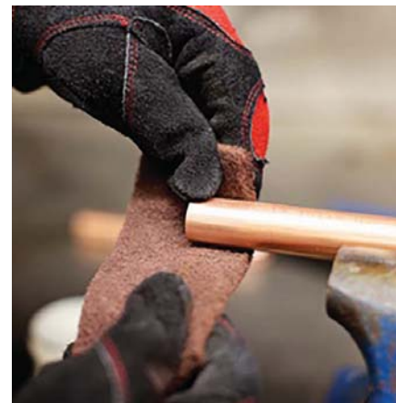
The joint surface areas must be clean and free from oil, grease, or oxide contamination prior to brazing.
