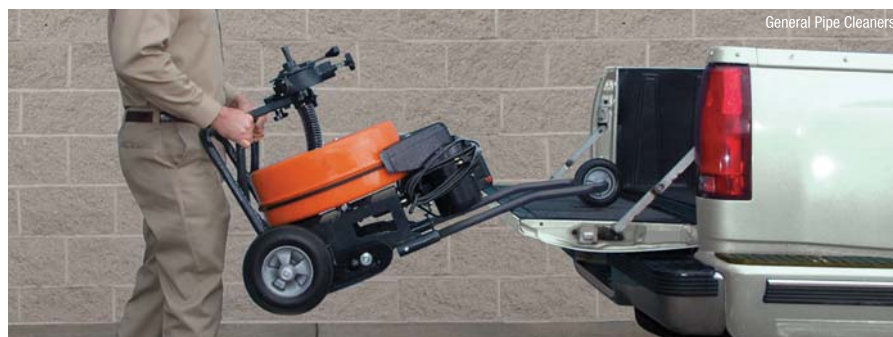
Compact size and portability can be important concerns when selecting a piece of drain cleaning equipment.
