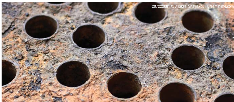
Mineral deposits, scale and corrosion on the plate of a heat exchanger.
