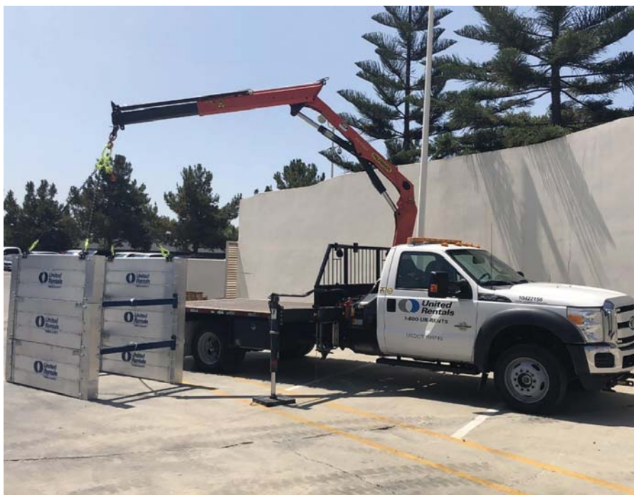
Spreaders should be used only to hold the box walls in place, not for pulling the box up or relocating it in any way.
